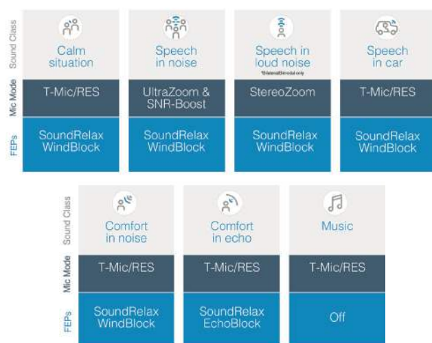
Figure 4: AutoSense OS 3.0 sound classes and associated microphone modes and front-end processing features (FEPs). Note that default strength settings for FEPs may vary by sound class.
